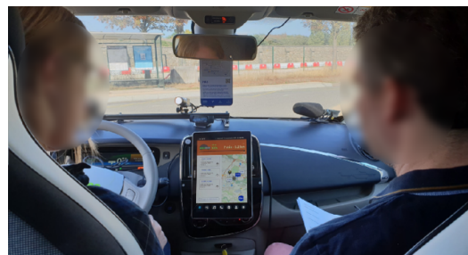
Figure 5: Integration of the personalised HMI framework and the central stack GUI application in an electric vehicle.
